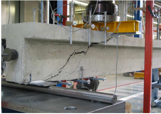
Figure 1: Experiments in Civil Engineering are limited, risky and costly; appropriate visualization can gain insight into aspects which are not visible in reality. Here we see a typical experiment of a structural concrete beam. Deep understanding of this processes are essential and form the basis for in-depth learning.
